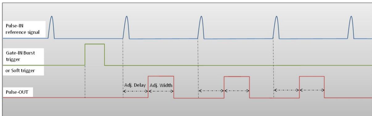
Figure 1 : Burst signal of 3 pulses, "Gate-IN" or Soft triggered and "Pulse-In" synchronized
